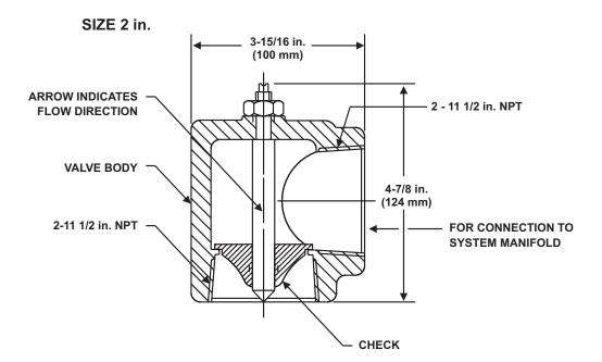
MATERIAL: VALVE BODY: ZINC PLATED STEEL CHECK: STAINLESS STEEL SEAT: NITRILE RUBBER
